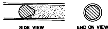
FIG. 4. Schematic representation highlighting the difference in catalyst action during channel propagation and filament gasification. In the latter situation, the particle can be considered as operating in a tunnel.
